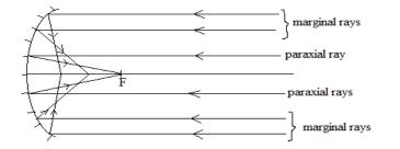
Rays close and parallel to the principal axis converge at F after reflection. When a wide beam of light is incident on a concave mirror, the different reflected rays are converged to different points. However these reflected rays appear to touch a surface known as a caustic surface (a
