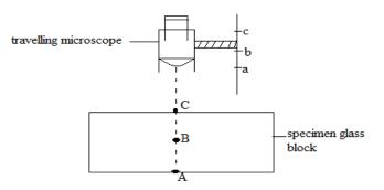
A cross is made on a white sheet of paper and the paper is placed under a travelling microscope.
