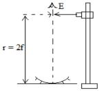
A concave mirror is placed on a horizontal table with its reflecting surface facing up. A pin is clamped horizontally on the retort stand such that its pointed end lies along the principal axis of the mirror.
