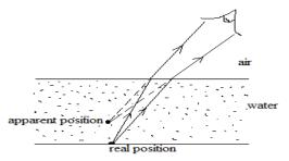
Light rays proceeding from an object at the bottom of the pond travels from water to air. After reaching the water-air interface, they are refracted away from the normal to the observer's eye. To an observer, the object (at the bottom of the pond) appears to be in the same straight line with the rays entering the observer's eye which makes it appear to be raised and the pond appears shallower than its really is.
