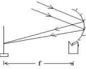
The setup is made in such a way that the concave mirror faces a distant object. The position of the screen in front of the mirror is adjusted until a clear image of the distant object is formed on the screen. The distance between the screen and the mirror is measured and recorded and it is the focal length of the mirror.
