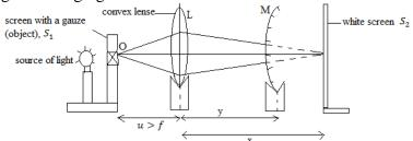
Without a convex mirror, M, the lens L is placed at a distance, u greater than its focal length.
