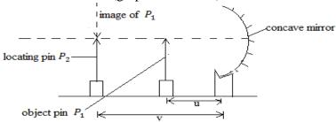
An object pin  $P_1$  is placed at a distance, u in front of a mounted concave mirror such that its tip lies along the principal axis of the mirror and it forms an inverted image.
