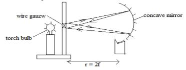
An object in this case consists of a cross wire in a hole on a white screen. The wire gauge (object) is illuminated from behind by a source of light A concave mirror mounted in a holder is moved to and fro in front of the screen until a sharp image of the cross wire is formed on the screen adjacent to the cross wire (object). At this point, both the image and the object are at the same distance from the mirror hence both are at the centre of curvature
