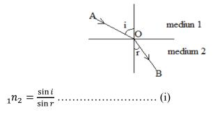
If the light source is altered so that it moves from B to O, then applying Snell's law,
