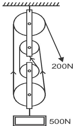
Given that the size of the load is 500N and the effort applied is 200N, calculate the efficiency of the machine. (3 marks)
